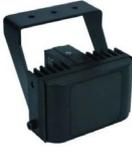
IR Strahler 940nm   short range   wechselbarer Abstrahlwinkel/Reichweite:<br>10°/95m, 20°/57m, 30°/46m, 60°/28m, 80°/21m, 95°/14m   12-32VDC oder 24V AC   13W      | A 1A            | 292,38           |
